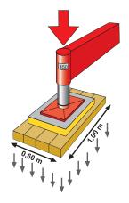
Ground pressure at 0.6 m<sup>2</sup> can be up to 750 kN/m<sup>2</sup>.
